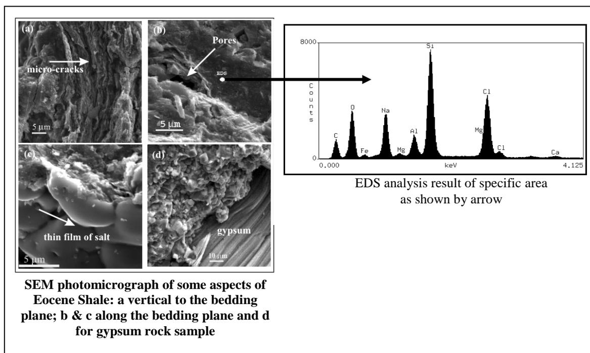
**Figure 7. SEM photomicrographs and EDS analysis of shale samples from District No.17, 15<sup>th</sup> of May City.**
